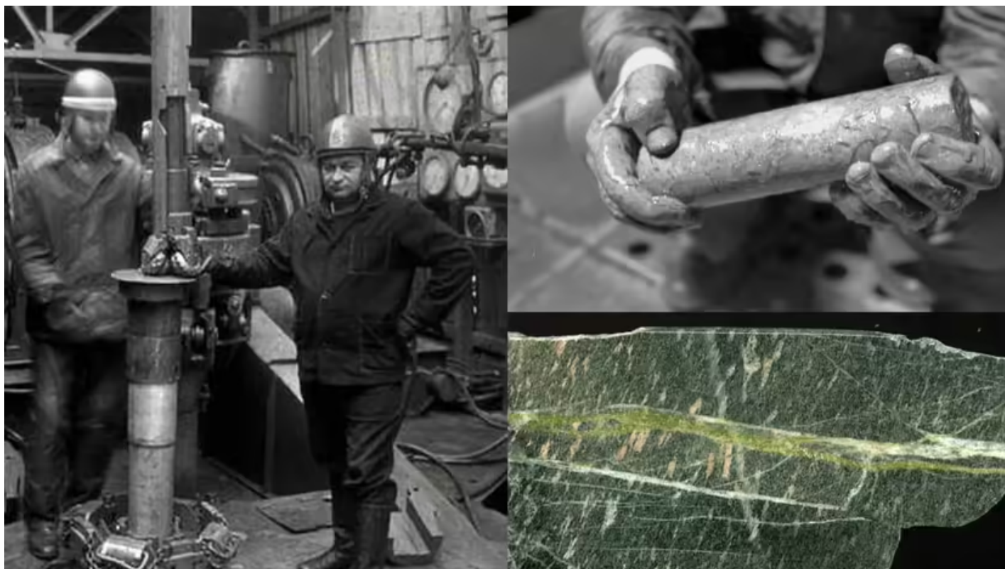
(Clockwise from left) Workers in the drill room; a piece of core extracted from the Kola well; a piece of metabasalt rock from 6,238.25 meters (20,465 feet) deep in Earth's crust. PECHENGA
