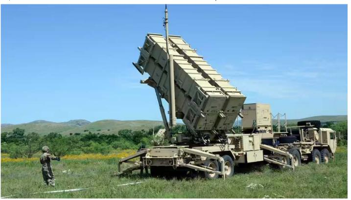
Patriot missile launchers can hold between four and 16 missiles, depending on the type. U.S. ARMY
